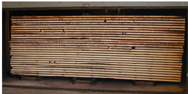
The Hodges Wood Products Lab's steam heated lumber dry kiln has a capacity of 1000 board feet
