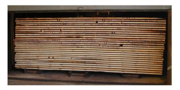
The Hodges Wood Products Lab's dry kiln has a capacity of 1000 board feet and is an updated steam lumber dry kiln with computer controls.
