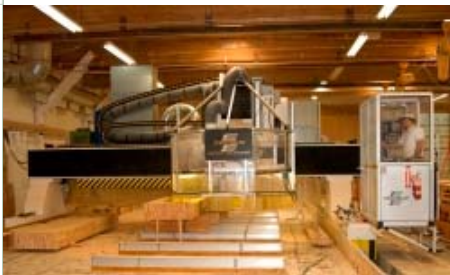
Engineered wood products are dimensionally stable, with predictable shrinkage, so machines like the ones used by Structurlam can cut them within extremely tight tolerances.
